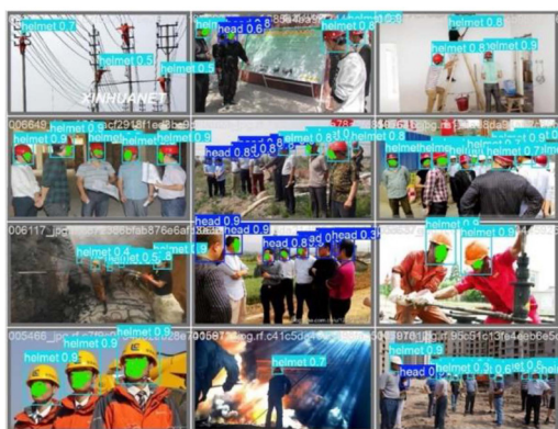
Fig. 6 Example output from the YOLOv11n model detecting individuals wearing and not wearing helmets. To protect personal privacy, certain details in the image have been censored.
