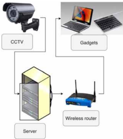
Fig. 2 Conceptual illustration of a CCTV camera system, adapted from A. Kurniawan et al. [10].
